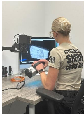
CSI Savannah MacLellan analyzes a fingerprint using the Full Spectrum Imaging System II.
